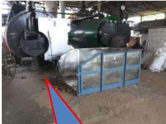
Install material handling system for semi automatic feeding of fuel
